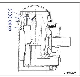
5. Use torque wrench to tighten the screws of cover (2) to the specified torque.
