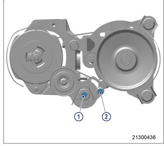
3. Tighten screw (2) with torque wrench to the specified tightening torque.
