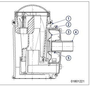
6. Use torque wrench to tighten the screws of cover (4) to the specified torque.
