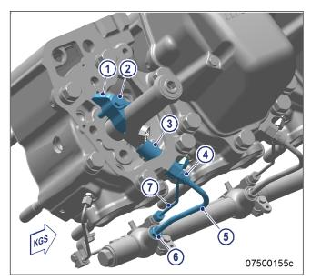
10. Fit hold-down clamp (1) in the correct position and use torque wrench to tighten screw (2) to the specified initial tightening torque.
