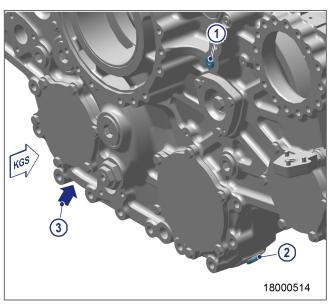
6. Tighten drain (2) and (3) with torque wrench to specified tightening torque.
