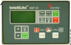
Electronic control unit and a programmable microprocessor, LCD display with backlight Off/Auto/test controls, Display of all parameters of the engine and alternator. Diagnostic information of the gen set, Automatic and manual control of the contactors, Mains voltage (on 3 phases), gen set voltage (on 3 phases), 3 gen set current, mains and gen set frequency, RPM counter, Vdc Battery, D+Voltage, KW-KVA-KWh – cosfi average.25 alarm messages and 9 pre-alarm.
