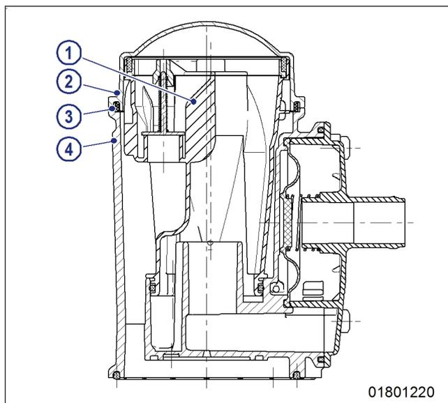
5. Use torque wrench to tighten the screws of cover (2) to the specified torque.
