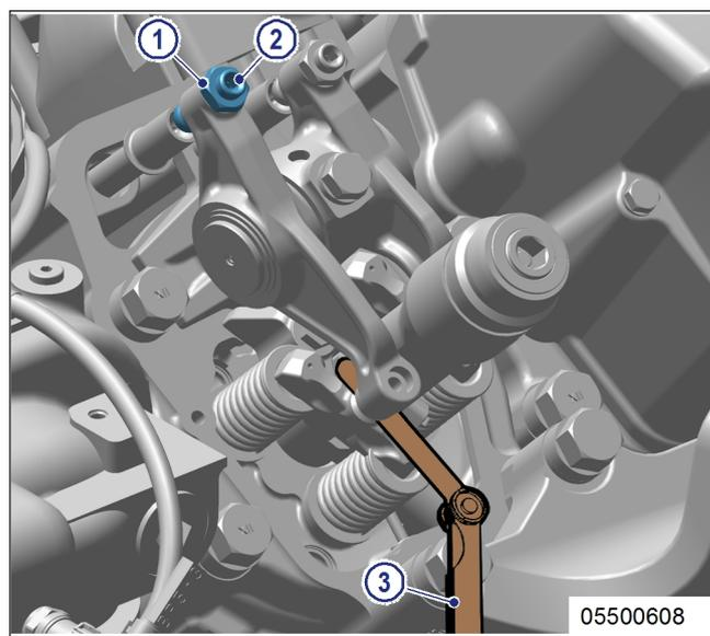
5. Tighten locknut (1) with torque wrench to the specified tightening torque, holding the adjusting screw (2) to prevent it from turning.
