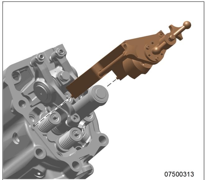
9. Remove sealing ring (4) from injector or use a self-made hook to take it out of the cylinder head.
