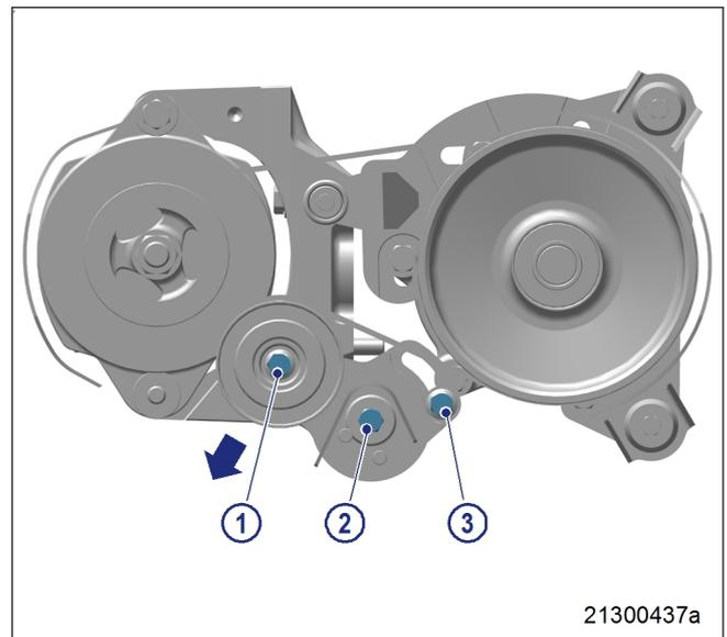
8. Tighten screw (3) to specified tightening torque using a torque wrench.
