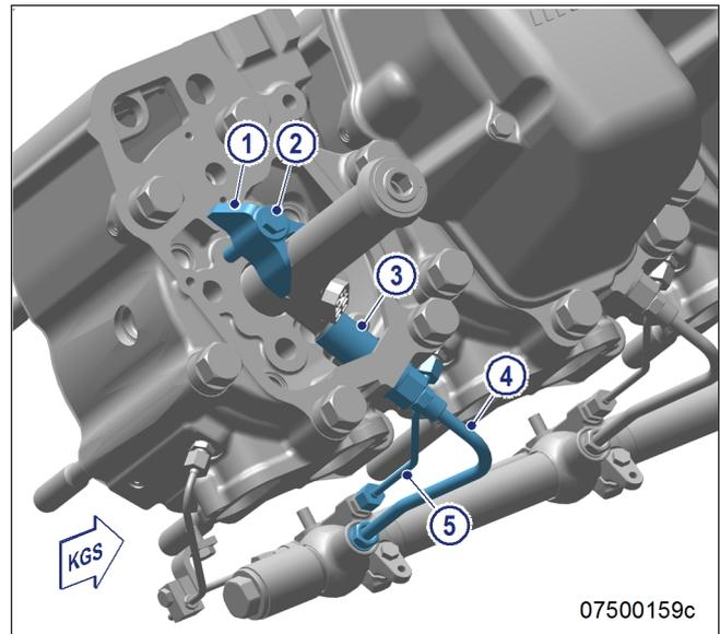
6. Install installation/removal tool on cylinder head.
