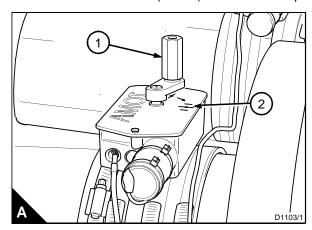
Note: Each air shut off valve has two positions. (A1) closed and (A2) open.
