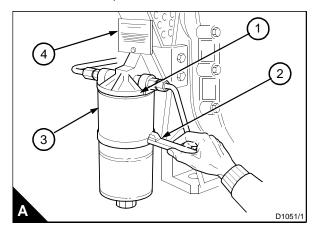
**Caution:** The plate (A4) contains information on how to drain the fuel filter canister. It also has information on when to change the filter canister. Before the filter is changed refer to the maintenance schedule.
