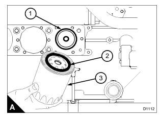
**Note:** After all the oil filters have been fitted, check that the air shut off valves are in the open position and prime the oil system, see "How to prime the engine oil system" on page 17. Do not start the engine.
