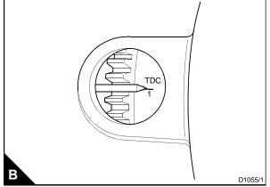
Note: Use the inspection hole (B) in the flywheel housing to find TDC number one and number six.
