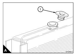
**Note:** After installation and before the first engine start, remove the radiator cap by rotating it anti-clockwise. Fill the cooling system with the required coolant. Run the engine off-load for one minute to ensure that the system is completely filled, then stop the engine and top up the system to 25 mm (1") below the top of the filter neck then replace the cap.
