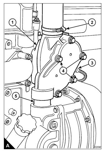
**6** Remove the two short setscrews which remain, separate the two halves of the assembly and remove the thermostats.
